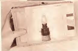
This is all there is to the retouching box. The film carrier is placed over the cutaway section of box.
